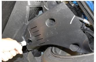
Remove the (3) 8mm hex screws retaining trailing arm splash guard.
