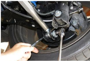
Now install outer NM Control Arm to trailing arm using factory bolt and adjusting plate. Line-up previous made pen mark before tightening. Torque to 100Nm (74ft.lbs).
