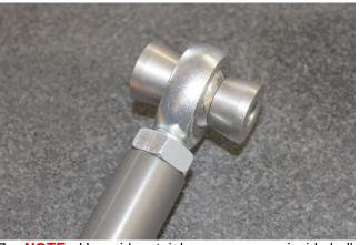
NOTE: Use wider stainless spacers on inside ball joint that attaches to sub-frame and the narrower stainless steel spacers on ball joint that attaches to outer suspension housing. The NM Control Arms have been pre-set to the factory length of 518mm (20.39").
