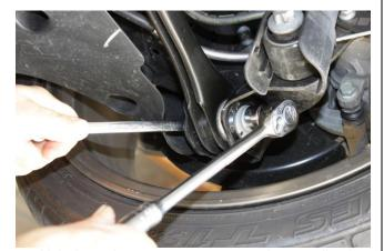
4. Unbolt and remove outer control are adjusting bolt. Hold bolt head with E14 Torx or 11mm box end wrench and turn nut with 18mm socket.
