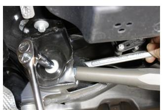
Install and tighten NM Control Arm into inner subframe mount using original bolt and nut. Torque to 100Nm (74ft.lbs).
