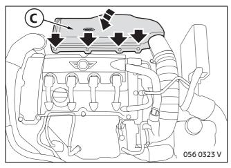
Fit air filter **C** on bottom of housing and secure as per TIS No. 13 71 000.
