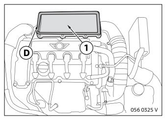
Fit seal **D** on bottom section of air filter housing (1).
