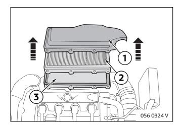
Remove the upper section of air filter housing (1) and remove filter element (2). The bottom section of the air filter housing (3) remains in the vehicle.
