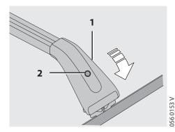
Swivel the cover cap (1) closed and close the lock (2) with key **B**.
