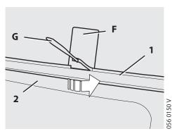
Push fitting aid F between the roof strip (1) and the roof (2). Carefully pull off the pre-cut piece of the roof strip with detachment aid G.
