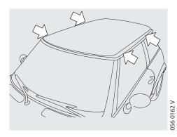
There are mounting fixtures at four locations on the roof for fitting the roof luggage rack. 4
