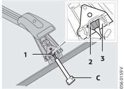
Tighten the bolt (1) until the two arrows on torque wrench  ${\bf C}$  lie above one another. This indicates the required torque of 6 Nm is reached.
