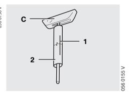
There is a line (1) on torque wrench C. This serves as a positioning aid when sliding on the lower sleeve (2) if it has become loose.
