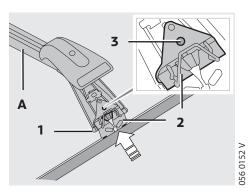
Carefully place the feet (1) of roof luggage rack **A** on one side according to the alignment instructions on the bottom of the profile on the roof.
