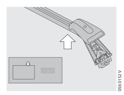
At the bottom right of the roof luggage rack profile there is a label which shows the alignment of the roof luggage rack on the vehicle roof.
