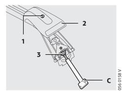
Open the lock (1) and swivel the cover cap (2) upwards.
