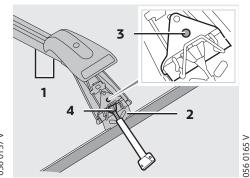
Install cover cap **D** in the mounting fixture (1).
