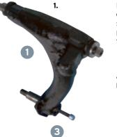
Radius arm for vehicles with dampers (known as dry suspension shock absorbers). Complete with pins and necessary parts ready to fit.
